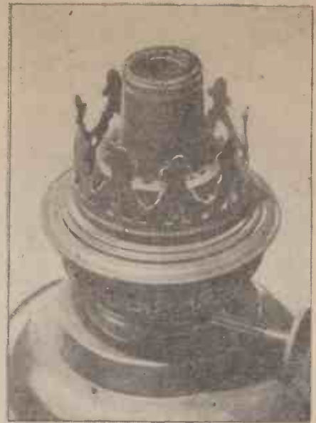
A close up view of a tubular wick burner constructed on Argand's principle.
