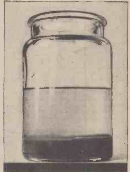
A piece of solid cake glue after immersion in cold water gradually absorbs the water and slowly swells, becoming a formless mass of mixed water and glue particles, which disperse into a clear colloidal solution on heating the liquid.
