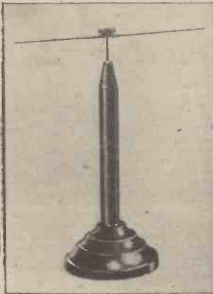
The pivoted magnetic needle, the properties of which Dr. Gilbert used for his investigations. Note the dip of the needle.
