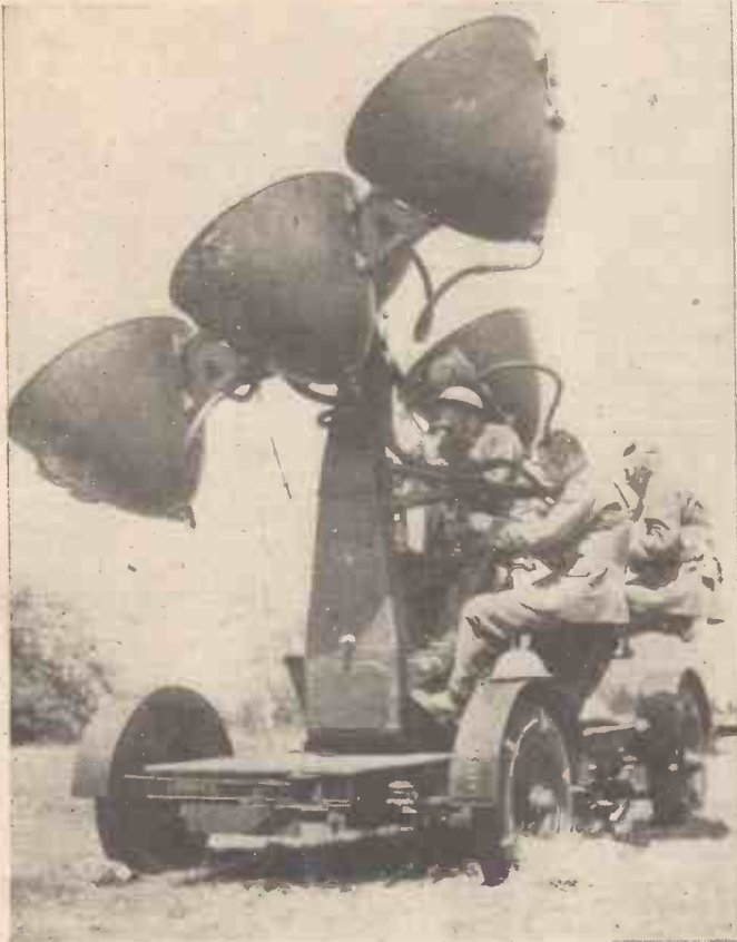
A sound-locator, with its crew of three, at an anti-aircraft station somewhere in England. One man works the course-finding bowl, whilst the other two listen-in on the large sound detectors.
