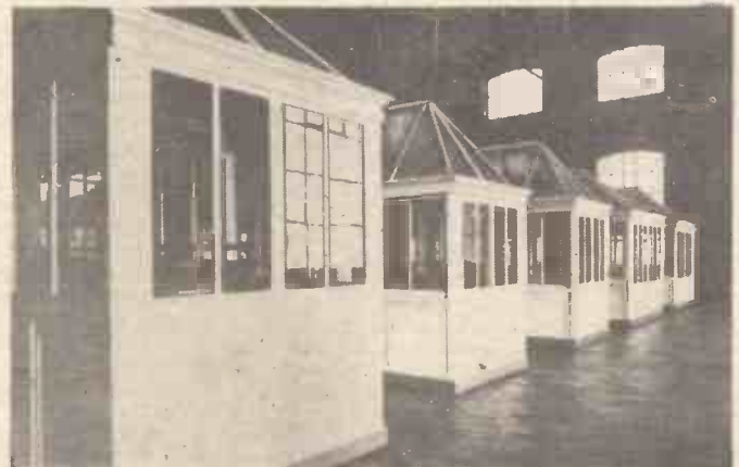
Heavily lead-lined processing booths in a radium factory. In these isolated apartments radium salts are progressively concentrated by chemical means.
