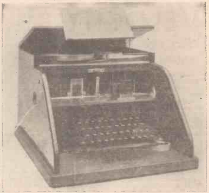
By courtesy of the Postmaster-General. The Gell perforator telegraph instrument of 1906.
