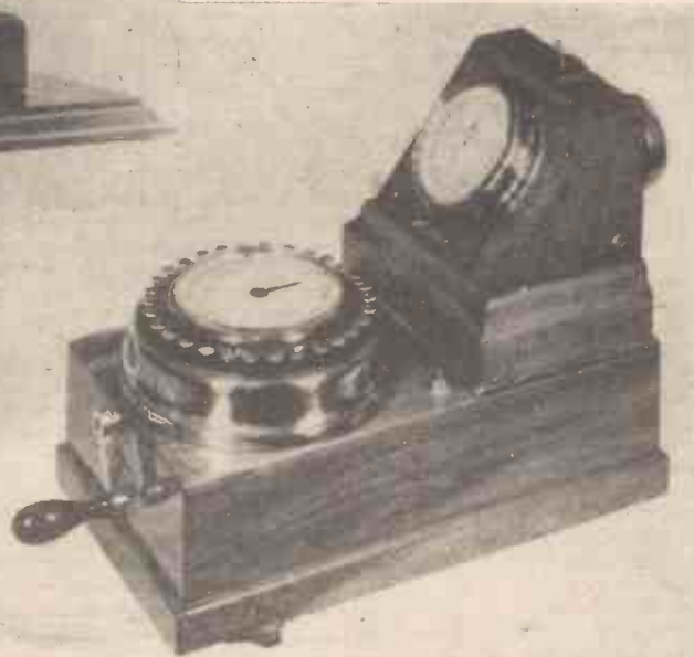
(Left) Wheatstone's ABC "step-by-step" transmitter as used about 1839. (Below) Wheatstone's ABC telegraph instrument — about 1840.
