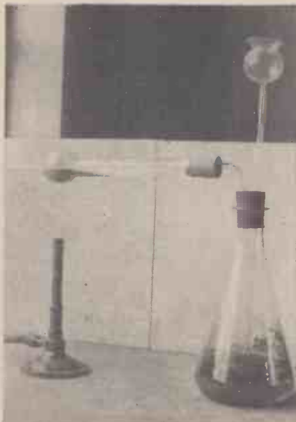
Making calcium hydride by passing a stream of hydrogen gas over heated metallic calcium.
