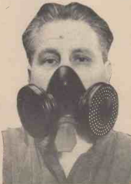
This is not the latest type of gas mask for use in air raids, but is a dust protector for use in dusty factories, or for work where the air is impure. It is one of the many safety devices produced by members of the Home Office Industrial Museum.
