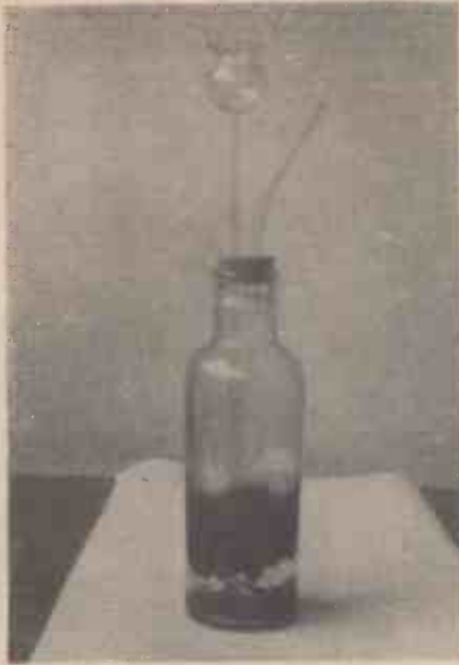
Apparatus for generating hydrogen. The bottle contains scrap zinc (or iron) and sulphuric (or hydrochloric) acid.
