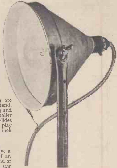
Fig. 1.—The funnel reflector attached to the upper end of the narrower tube.
