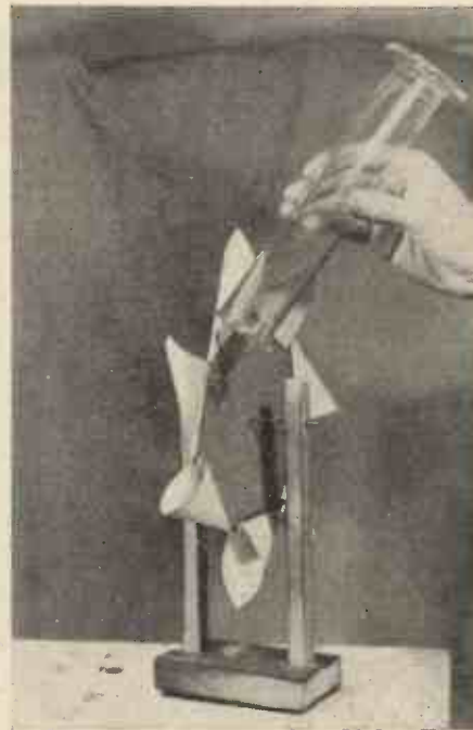
The carbon dioxide wheel. The carbon dioxide gas is "poured" from the glass jar into the paper cups on the edge of the wheel. Being heavier than air, it fills the cups and weighs them down, thus setting the wheel in motion.
