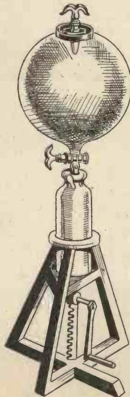
Boyle's original air-pump, the first mechanical air-pump to be made in this country.
