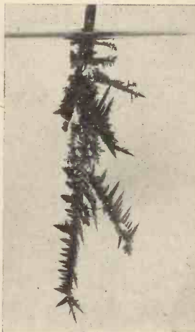
A "lead tree." It is composed of crystals of metallic lead.
