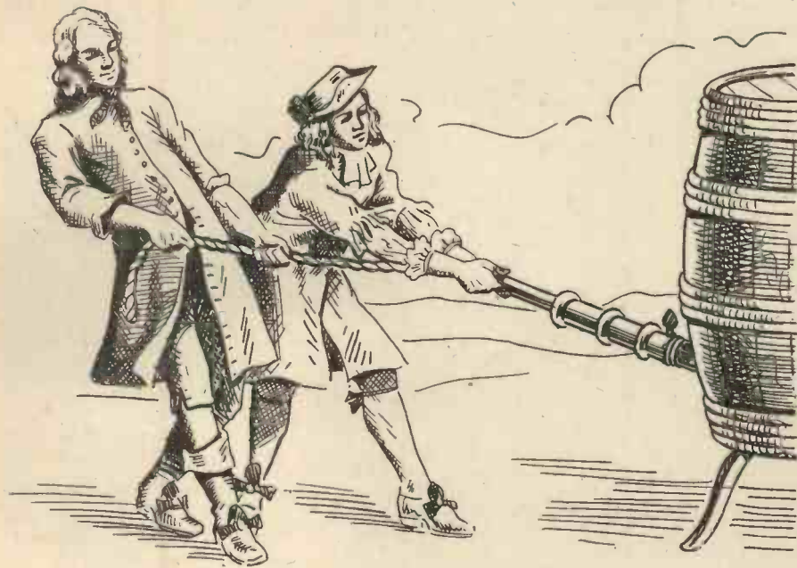
An early air-pump experiment to remove air from a sealed barrel by means of a crude type of pump.
