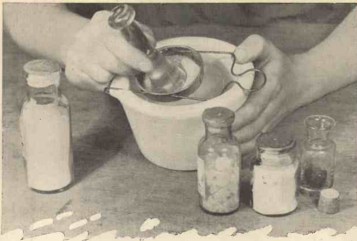
Grinding the heat-indicating material through a wire sieve in the preparation of the heat-sensitive paint.
