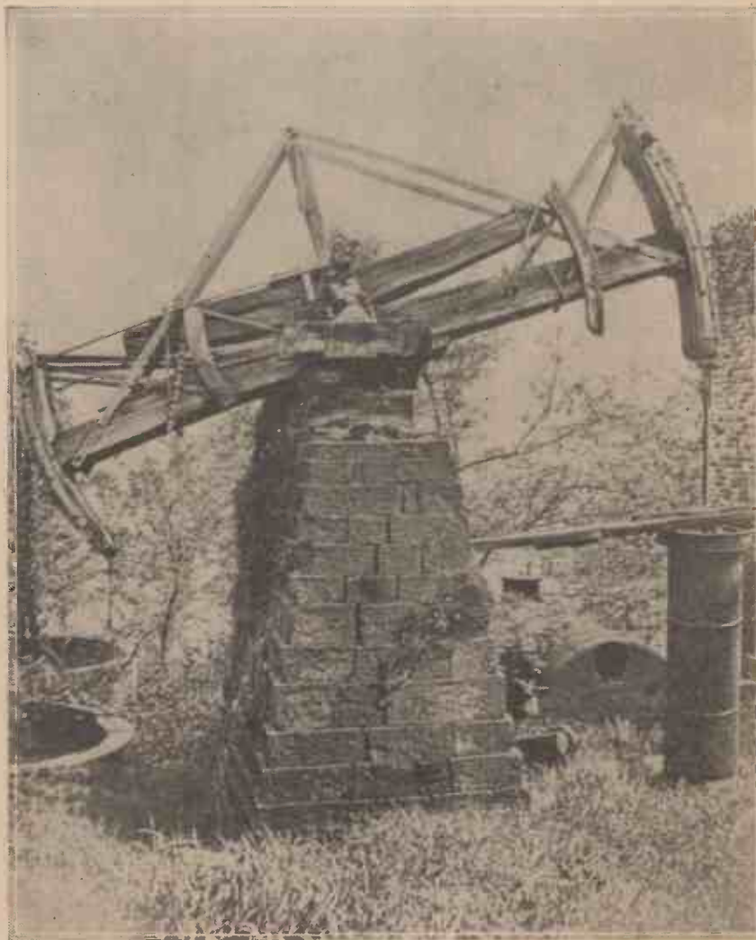
Probably the last-remaining Newcomen engine in this country. For many years it stood in a field near Ashton-under-Lyne, Lancs, before being purchased as a relic by Mr. Henry Ford and being shipped to America.
