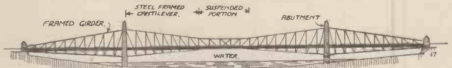
Fig. 17.—A steel-framed cantilever bridge, as used for very large spans. Our Forth Bridge was constructed on this principle.
