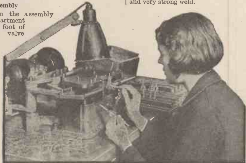
Assembly Detail: Bending the supporting wires accurately to size and shape to receive the electrodes.
