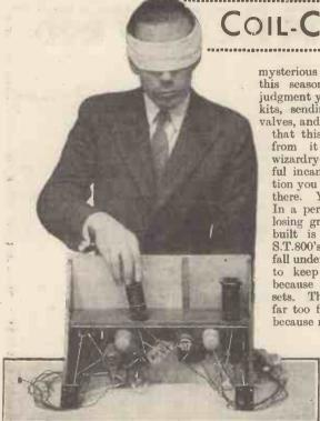
The new self-locating coils used in the S.T.900 are so simple to fit into their holders that this can be done blindfolded with perfect certainty that they can be immediately Inserted. Coil-changing takes only a second or two.
