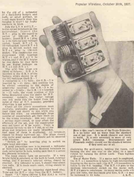
Here is this year's version of the Triple Extractor. It is no better and no worse than the standard one of last year. It is much cheaper and easier to build. It is only necessary in cases of very severe B.B.C. swamping. Bournemouth and Plymouth readers should use the standard version if they need any at all.
