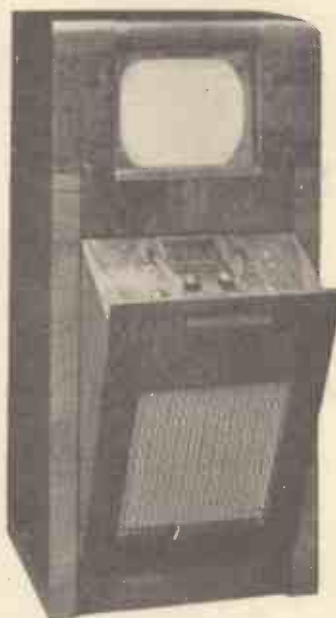
Access to the all-wave-radio controls on this Baird instrument is obtained by tilting the front panel as shown.
