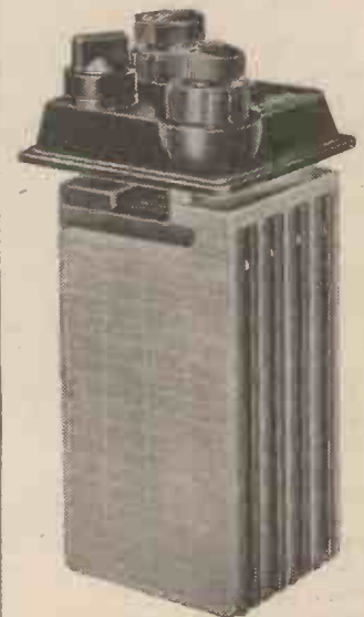
The latest Exide "Hycap" G.F.G.4-C cell (24 amp. hours). Compare it with the "Mass" type. Note the decreased thickness of the plates and the increased number. These cells will give a bigger current output and can be recharged more quickly than the "Mass" type.
