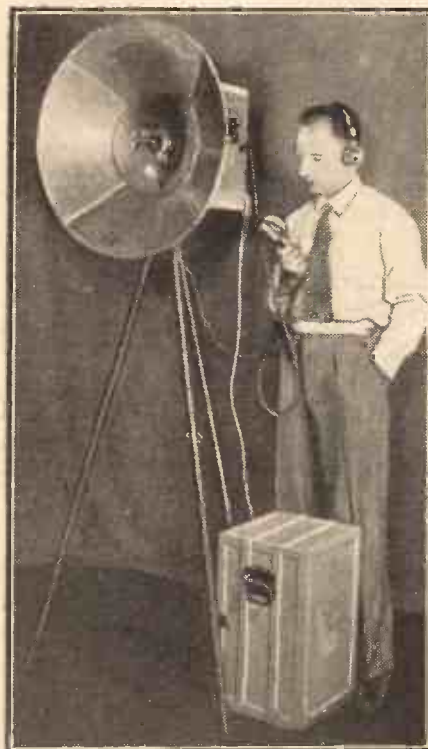
A combined Telefunken micro-wave transmitter and receiver for two-way communication. The aerial is in the centre of the reflector, and is used for both transmission and reception.
