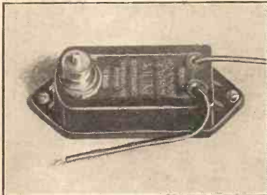
Here is a different kind of trap—one for the noises that get into a wireless set from the mains. It is the Graham Farish "Mum" Suppressor.
