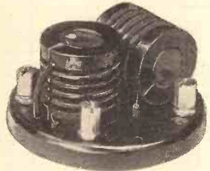
A neat wave-trap unit that has been specially designed by Wearite to cope with modern conditions.
