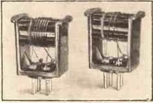
Attractive mounts with horizontal formers are a feature of these Colvern short-wave coils.
