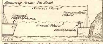
The sound-and-wireless method of obtaining accurate distance between a ship and the shore. The time between reception of the radio and the sound signal enables the distance from the transmitter to be worked out.
