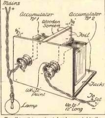
How the unit is constructed and connected to the electric light supply.
