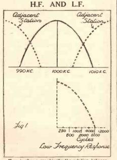
Here is shown graphically the relation between a tuning curve and the low frequencies with which the carrier is modulated.
