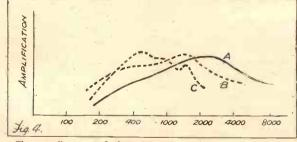
The overall curves of three different sets taken under working conditions. C has little bass and no "top"; while A has fairly good "top" but a bad falling-off at the bass end. B has the best "balance."
