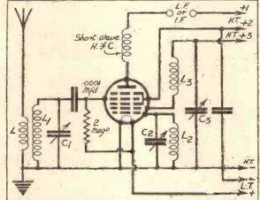
How a heptode valve is connected up to work as oscillator and \_\_\_\_\_ mixer in a short-wave superhet.
