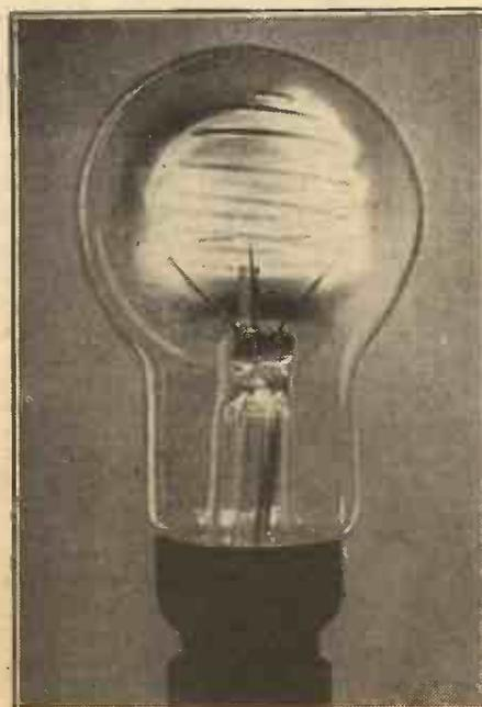
The neon lamp is a practical example of an electron discharge producing a luminous effect.
