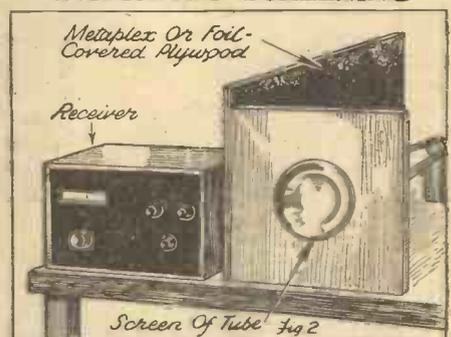
The tube and time-base apparatus should be well screened from the receiver if these two sections are placed fairly close.
