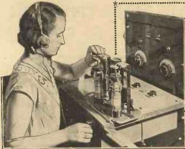
Coil-testing in progress in the Coscor factory. Every coil is tested many times, to ensure correct electrical characteristics and for mechanical soundness.
