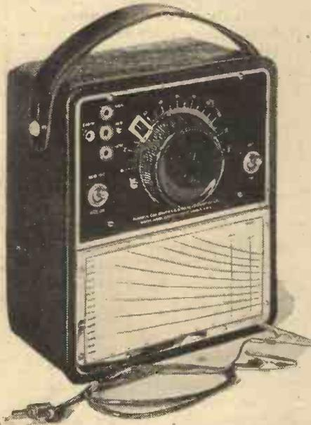
Though not an essential instrument, a calibrated oscillator such as the above is very helpful for such work as condenser ganging.
