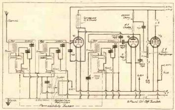
The six "variable condensers" shown across the coils in this diagram are the trimmers and are incorporated in the coil unit. Once set they do not have to be touched. The long-wave and medium-wave inductances are separately trimmed, as was explained last week.
