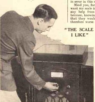
Typical of good modern condenser-scale design is this wide-vision, wave-length-calibrated scale used by Mr. Scott-Taggart in his famous "Super-Gram de Luxe." It has 10-metre markings on the medium-wave side.
