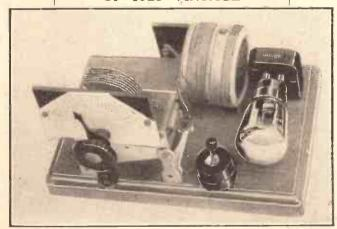
This interesting short-wave receiver, to which W. L. S. refers in the article on this page, was built in 1923. Note the "low-loss" coil, horizontal valve mounting and calibrated dial.
