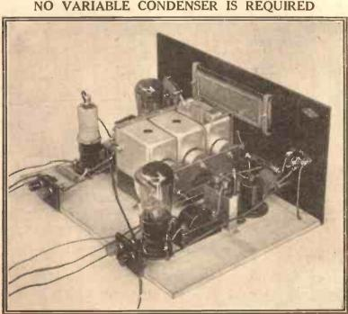
A general view of the "Nu-Tune" Three. Note the iron cores which slide in and out of the coil centres, controlled by the tuning knob on the panel.
