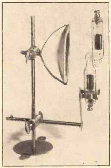
The "T.I." lamp, with its stand and reflecting mirror. The pictures obtained with this outfit are much brighter than those given by an ordinary neon-tube light source.
