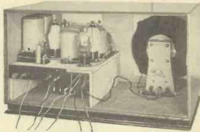
A back view of the All-Wave Four-Valve Superhet with the batteries removed to show the loudspeaker. Note the two condensers, value .002 mfd each, across the terminals of the loudspeaker.
