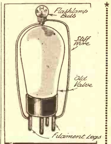
A burnt-out non-metallised valve is used for this scheme. The glass bulb makes the insertion of the tester an easy matter.
