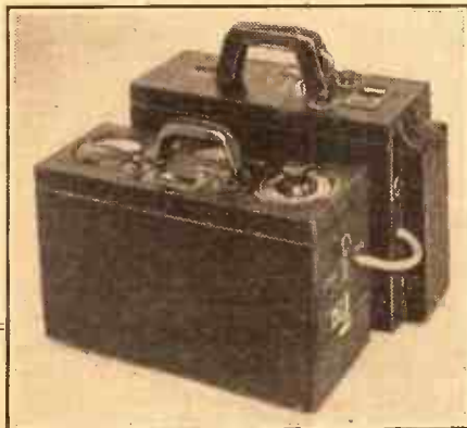
Electrical interference, from all sorts of machinery and even motor-car ignition, is specially noticeable on short waves. The photograph shows apparatus that would delight the short-wave fan—a Siemens interference-detecting set which permits of complete portability.
