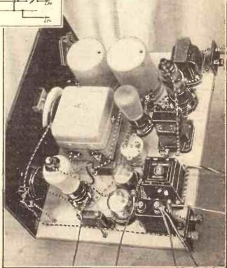
The S.G. valve is the one in the toreground. The valve near the coils with the anode cap being the new driver-B amplifier.
