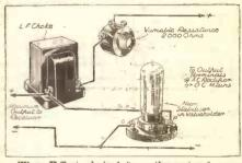
When H.T. is derived from the mains for a Class B receiver, it is advisable to use a voltage stabiliser across the mains unit as shown.
