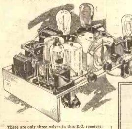
There are only three valves in this D.C. receiver, the fourth "valve" (second from the left) is the vacuum barretter that controls the heater current.
