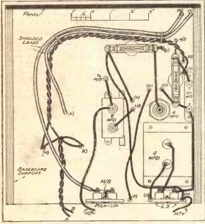
The screened leads and the twisted dek heater connections run mainly below the wooden baseboard, which is sprayed with metal to form a screened chassis.
