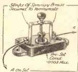
When the condenser is screwed to the knob shorts the two metal strips.
