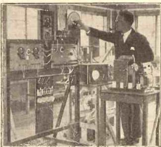
The picture on the left shows part of the 3-kw. transmitter which was taken north for the experiments, while Mr. Geoffrey Builder, Professor Appleton's chief lieutenant, is seen above with the cathode-ray oscillograph and recording camera.
