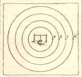
Fig. 1. The waves radiated from a broadcasting station get weaker as their distance from the transmitting aerial increases. Thus the strength of the waves at "a" is greater than at "b" and much greafer than at "c" and "d."
