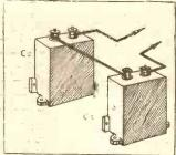
When condensers ary icined in series the resultant value is given by the formula  $\frac{1}{2}$   $\frac{1}{2}$  where by the formula  $\frac{1}{c} = \frac{1}{c^1} + \frac{1}{c^2}$ C is the total capacity.
