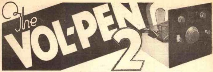
Power and selectivity are combined to an amazing extent in this compact all-mains two-valve receiver. It makes use of one of the latest and most efficient pentode valves, and is capable of an output wattage of over 3,000 milliwatts.
