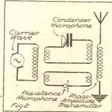
Fig. 2 (seen above) shows a typical experimental dual transmitter. Phase modulation is applied through the condenser microphone and amplitude modulation through the resistance microphone.
