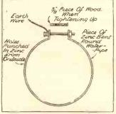
Obtaining a good water-pipe earth will be assisted by this clip.
