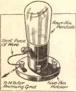
The flex lead ‡ enables side-terminal centodes to be used in addition to the 5-pin variety.
