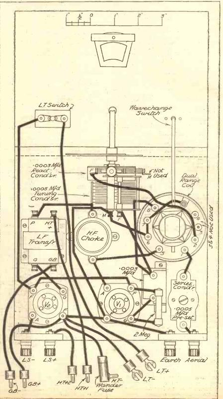
This wiring diagram shows in an exceptionally clear manner the few connections that have to be made in the Unity Two. The reaction condenser unit is situated between the tuning condenser and the panel.
