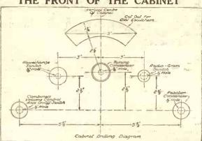
The cabinet front is drilled according to this sketch, dimensions being taken from the centre component—the tuning control. It desired, the cabinet can be obtained ready drilled.
