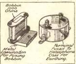
Old loudspeaker and headphone bobbins can be used very effectively as fixed resistances where small currents are being dealt with.
