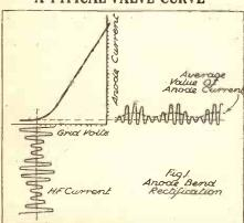
This is the grid-volts/anode-current curve of a valve suitable for anode-bend rectification. For best results the grid bias should be adjusted so that the operating point talls on the bottom part of the curve.
