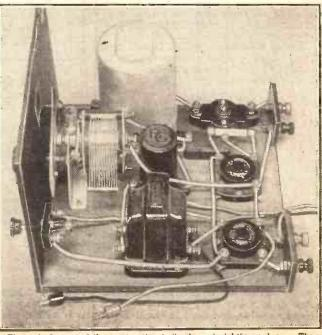
The main feature of the construction is its sheer straightforwardness. The two wander-plugs in the foreground plug into the grid-bias battery, which is accommodated on the side of the cabinet.
