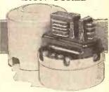
Iron-cored coils are the most recent development in tuning technique. Amongst other advantages, a big saving of space is obtained, as you can see by comparing this photo-graph with that of an air-cored coil of a similar type.
