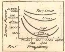
This diagram shows how reproduction varies with volume. If a 1,000-cycle note were produced by an intensity which made it just audible, a 50-cycle note would require a million times that intensity to make it equally audible!
