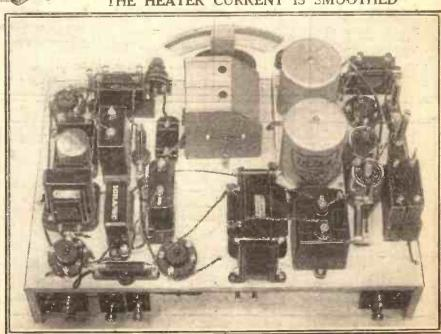
The large choke in the centre foreground is for smoothing the heater supply, and is essential to hum-free operation of the set.
