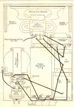
The Power Pack for the "Double X" also contains the loudspeaker and fits in the cabinet beside the chassis. It is best to connect up the two sections before they are pushed right into the cabinet.
