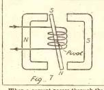
When a current passes through the coil in the direction shown, the top of the armature becomes a S. pole. Therefore, as unlike poles attract, the armature swings over to-the left.
