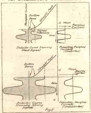
An interesting comparison between the effect of a weak and a strong signal on a detector which has a bottom bend is provided in this diagram. It will be noticed, as pointed out by P. P. E. in the accompanying article, that, while the ontput from the weak signal is somewhat distorted, that from the strong one remains comparatively unaffected.
