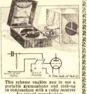
This scheme enables you to use a portable gramophone and pick-up in conjunction with a radio receiver for record reproduction.
