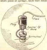
Here is an easily made wander plug socket which has many uses.
