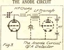
The anode circuit of a valve includes everything which is in the path of the H.T. current on its way from the anode through the H.T. battery to the cathode.
