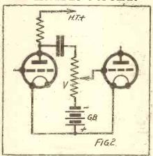
A favourite method of controlling volume on the L.F. side of a receiver is to employ a potentiometer as the grid resistance in an R.C. coupled stage.
