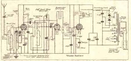
The circuit responsible for the astounding results of the A.C. "Double X." It has a screen-pentode H.F. valve and a specially sensitive output pentode. The two 4-mid. condensers in parallel between the smoothing choke and H.T.— were chosen instead of an 8-mid. in order to ensure easy availability.
