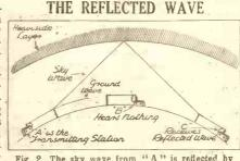
Fig. 2. The sky wave from "A" is reflected by the Heaviside Layer and picked up by "C." But "B" hears nothing because he is not in the path of the reflected wave or within range of the ground wave.
