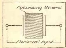
If a beam of polarised light is passed through the mineral, the momentary strains imposed upon it by electrical forces on the side plates will result in the beam being rotated.
