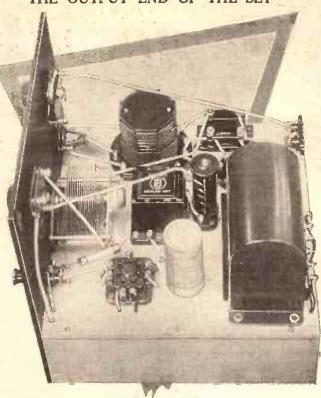
The output valve has a seven-pin base and needs one of the new seven-socket valve holders. The output choke, on the right, is of the tapped variety, and should be "adjusted" to suit the loudspeaker:
