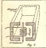
The soft-iron armature is mounted centrally between the two magnets and it is free to move about a pivot.
