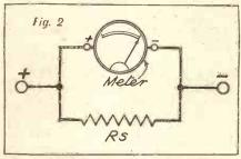
By varying the value of the resistance Rs the meter can be made to read up to 1 amp. The smaller the resistance the larger the current which can be read by the meter.
