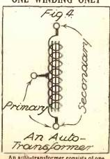
An auto-transformer consists of one winding only, different ratios being obtained by arranging suitable taps.
