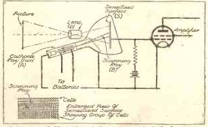
A diagrammatic illustration of the arrangement of the Iconoscope cathode-ray tube and its associated circuit as applied to the transmission of television pictures.
