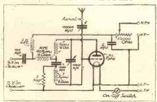
Here is a suggested circuit for a superhet adaptor covering the 5 to 7-metre waveband. It is suitable for attaching to an ordinary S.G broadcast receiver.
