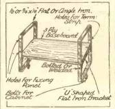
A set built on this type of chassis is particularly accessible.
