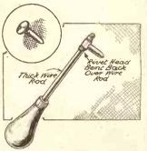
A really small soldering iron is a great asset. The one shown above can be made by anyone from a few odds and ends.
