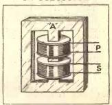
The core of a commercial transformer is made up of a number of laminations clamped tightly to-gether and insulated from one another.
