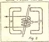
If the direction of the current through the coil is reversed, the upper end of the armature becomes a N, pole. Like poles repel, so the armature swings over to the right.
