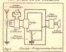
This receiving circuit includes a local oscillator and a filter. In practice these are arranged, so that they can be cut out so as to convert the set into an ordinary "straight" receiver.
