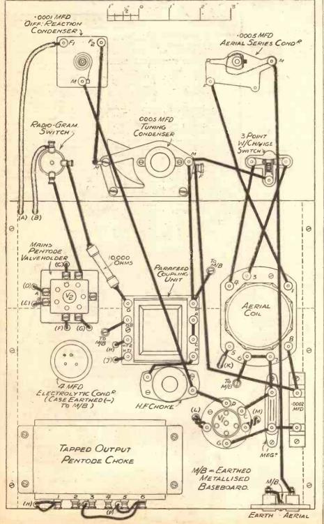
Besides the components shown on this above baseboard diagram there are a few situated below. This form of layout greatly simplifies construction, and makes for ease of wiring.
