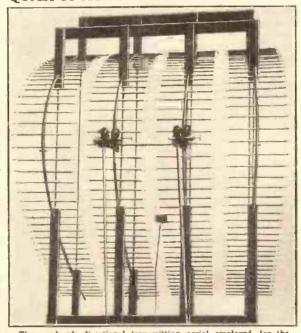
The quadruple directional transmitting aerial employed for the Marconi system of short-wave radio telephony on a wavelength of 50 centimetres, or 60,000,000 cycles per second!
