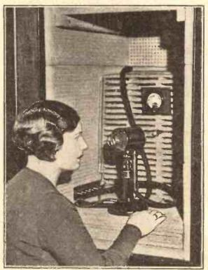
A condenser-microphone telephone transmitter at the Dollis Hill laboratories of the G.P.O. It is housed in a specially lined nonreverberating cabinet.
