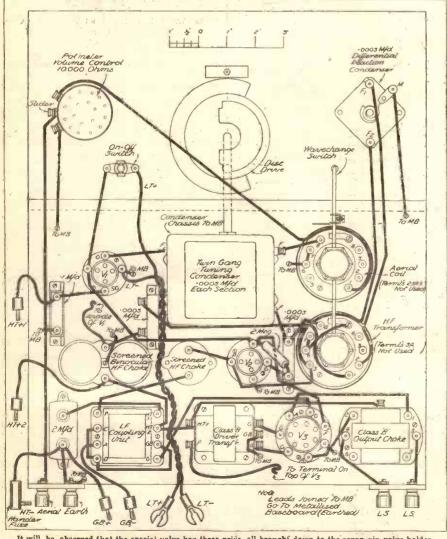
It will be observed that the special valve has three grids, all brought down to the seven-pin valve holder. Care must be taken that the right connections go to these terminals. An interesting feature of the new driver-B is the fact that it has three anodes as well.
