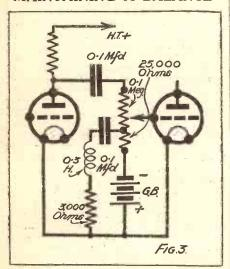
If the usual L.F. volume-control potentiometer is modified by the addition of inductance and capacity, as shown here, a better tonal balance is maintained when volume is lowered.
