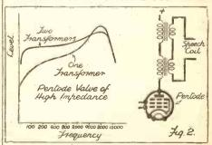
Showing how you can get more bass by using a higher anode impedance in the form of two transformers in series, as shown, provided the valve has a high impedance.
