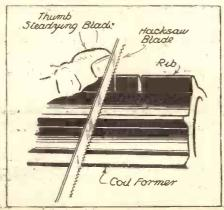
The slots are widened by making a second cut with the hack-saw, at the side of the first one.
