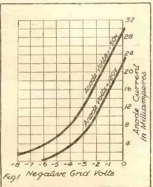
from the characteristic curves of a low-frequency valve (shown above), it is possible to find the correct grid-bias voltages for different high-tension values
