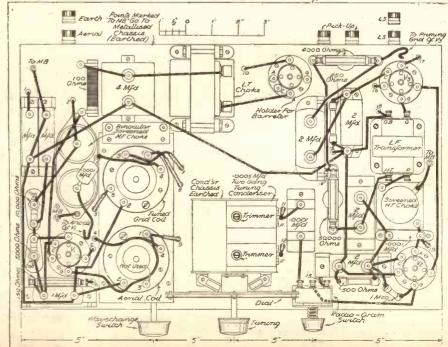
Most of the layout and wiring is carried out on the upper side of the chassis. The coil unit is raised by two small pieces of Metaplex so that the wavechange-switch knob is level with that of the radio-gram switch The coil unit is raised by two
