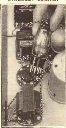
The driver B is a remarkable example of compactness in valve design. It is smaller than most Class B valves in spite of the fact that it contains a complete triode between the two "B" sections.
