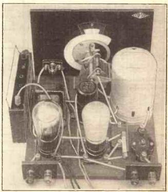
The tuning and reaction controls are carried out by concentric knobs on the main condenser. The screened coil reduces the danger of direct pick-up of a local station by the tuned circuit-of the receiver.
