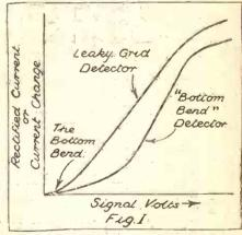
The bottom bend of a typical valve characteristic is shown in the diagram above. The curve on the last represents leaky-grid detection, while the other shows anode-bend rectification:
