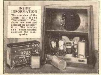
pentodes in quiescent push-pull. volume from batteries! And so that the ship shall not spoil for a ha'porth of tar, a special moving-coil speaker has been designed so that a fine output shall ensure even finer reproduction. Nothing is lacking on the score of quality.
