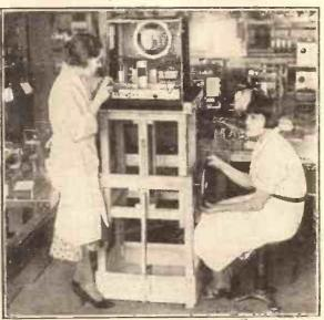
The most up-to-date production methods are employed at the H.M.V. factories at Hayes. Receiver assembly is greatly facilitated by the use of a special form of lift which enables the worker to reach every part of the set without undue fatigue.
