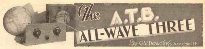
HE object of this set is to provide firstclass results over the whole gamut of useful wavelengths, from 15 metres to over 2,000 metres.
