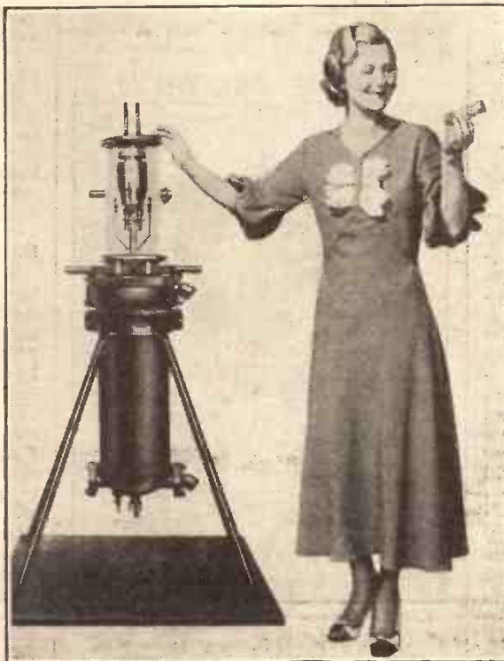
This is the Osram "Catkin" valve which travelled by post from London to Aberdeen and back exactly as shown without any protective covering! On arrival it was plugged straight into a test receiver, where it behaved perfectly, there being no trace whatever of internal damage in transit, although the valve had received a buffeting sufficient to bend one of the pins.
