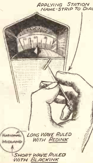
Mark the long and medium wave stations with different colours to distinguish them on the dial.
