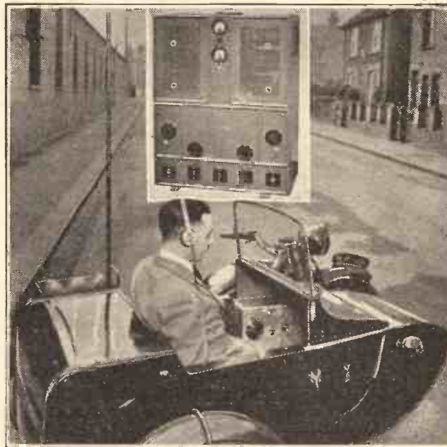
A radio-equipped motor-cycle combination to aid in the war on smash-and-grabbers. Inset shows the special Marconi transmitter to work at police headquarters, in conjunction with the mobile receiver. Notice the latter's rod aerial.
