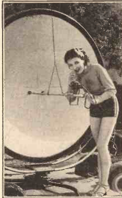
This parabolic reflector concentrates the sounds arising in its path on to the microphone, but extraneous sounds are largely eliminated. The principle has been successfully used for both outside broadcasts and the making of "talkies."
