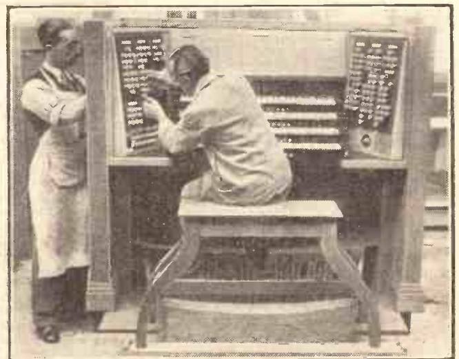
There are 2,362 pipes, and 149 electrical stops, some of which were being adjusted when this picture was taken.
