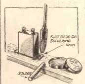
Obstinate screws soon give way to a hot iron and a " spot " of solder.
