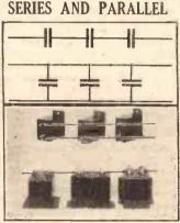
The top and bottom illustrations show condensers joined in series, and the centre pictures the parallel connections.
