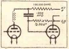
The value of decoupling resistances for R.C.C. stages should be half that of the anode resistance, provided this is not greater than 100,000 ohms.
