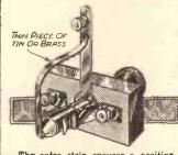
The extra strip ensures a positive instead of a "rubbing" contact on the third point.
