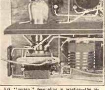
" screen " decoupling in practice--the resistance and condenser are arranged so that they come close to the screening-grid terminal in order to keep the wiring as short as possible.
