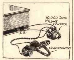
An arrangement which allows headphones to be used on the loudspeaker output terminals.
