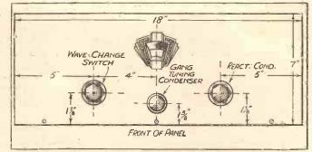
The main controls are mounted on the panel, the subsidiary ones being on the side of the cabinet.
