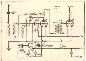
There are two panel lamps, one glowing red and the other green, according to the position of the switch, thus indicating which programme the set is tuned to.
