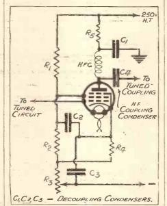
The circuit scheme recommended by the valve makers for their new H.F. Pentode. The resistance values are given in the table on this page.
