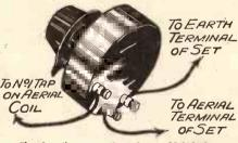
Showing the connections for a 10,000-ohm potentiometer as a volume control of the aerial input.
