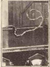
Instability is sometimes caused by the flexible leads from a loud-speaker or gramophone pick-up being allowed to trail over the top of the cabinet.
