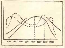
"The dotted lines show the frequency characteristics of bad speakers, giving unsatisfying quality! The full lines give characteristics of typical moving-iron speakers."
