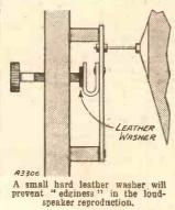
This metal-to-metal contact is very often the cause of a metallic "edginess" on heavy notes, and can be easily remedied by slacking off the adjusting pin and placing a small hard leather washer between it and the piece of spring steel, as in enclosed sketch. Incidentally, this will improve the tone of the speaker tone of the speaker.
