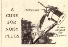
on the plug not being firmly held against the spring-loaded plugs in the liolder. This is often due to the bayonets being too near the end of the plug.
