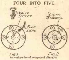
(it should have a resistance of about 50,000 ohms, by the way), and these terminals are connected like this.
