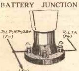
One side of each of the three bat-TOEARTH terjes is common.
