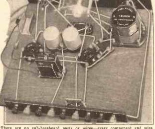
There are no sub-baseboard parts or wires—every component and wire is "above board."
