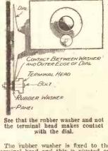
The rubber washer is fixed to the terminal head and this is pivoted on the panel so that the washer eugages with the outer edge of the dial. It can be fixed, in the same way with a complete an arrive between
