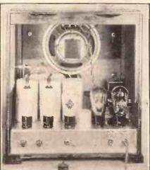
The magnetic system of the efficient loudspeaker is energised by mains current.
