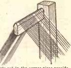
Slots cut in the corner piece provide simple spacing of wires.
