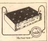
The positive terminal of a voltmeter should be connected to the positive terminal of the battery.
