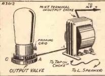
The loudspeaker lead should be tried on the different tappings provided to see which suits it best. (You should switch the set off before altering
