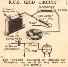
Anode resistance for R.C. coupled L.F stages : 100,000 ohms when employed in the first stage, and followed by a transformer.
