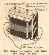
The number of turns necessary can easily be determined by winding on about twelve turns of No. 24 D.C.C. wire and adding or yemoving turns as required. The ends of the wire are con-nected direct to the dial lamp, which will light out outforthe line the other will light automatically when the set switched on.
