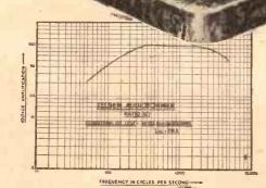
The excellent treble response secured can be seen at a glance in this graph showing the Telsen Audioformer curve.
