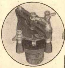
The Ormond differential reaction condenser modified for the "Airsprite "—an extremely easy task.
