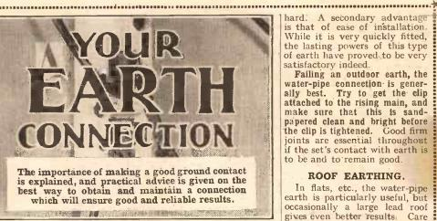
" biscuit-tin earths " are too | away, where the ground keeps small to be really efficient, but, on continually moist the other hand, the buried sheet of galvanised iron roofing, superexcellent though it undoubtedly is may prove too elaborate for your needs.
