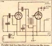
Parallel feed has the effect of increasing the transformer's primary impedance, because direct current is removed from it.
