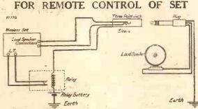
Plugging in the speaker automatically switches the set on.
