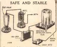
The usual S.G. connections and method of joining in the aerial through a 0001 fixed condenser.
