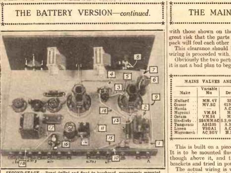
SECOND STAGE .-- Panel drilled and fixed to baseboard, components mounted, wiring commenced.
