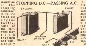
The two-mid. condenser in an output filter circuit has a double duty to perform: It keeps the anode current out of the speaker, and allows the speech currents to flow.
