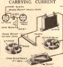
The resistance in the anode circuit, unlike the one in the following valve's grid circuit, has to carry a definite number of milliamps.
