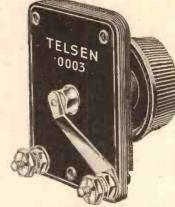
TELSEN AERIAI SERIES CONDENSER The ideal volume and selectivity control, solidly constructed, with very low mini-mum capacity. The externally keyed switch-arm when rotated to a maximum position, connects with a contact on the fixed vanes, thus short-circuiting the condenser for maximum volume. Supplied complete with knob. Capacity .0003
