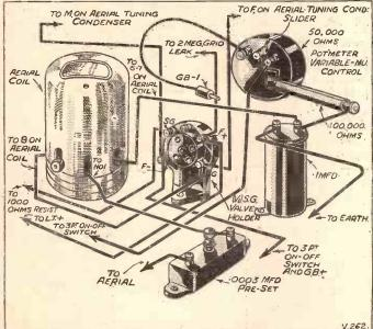
The arrangement used for the variable-mu control in the "Airsprite." Its use prevents H.F. getting through to the bias battery and causing instability and motor-boating. It is especially valuable when a mains unit is used.
