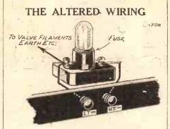
The correct connections for a fuse in the H.T. negative lead are very clearly shown here. There must be only one wire from the side which goes to H.T. negative, and that wire must go to the H.T. minus terminal. Every other lead, grid bias positive included, must go to the L.T. negative side of the fuse.
