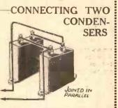
series or parallel. This is a convenient means of increasing or decreasing the total capacity should it be necessary to do so.
