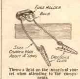
L.T.-, that is, when the accumulator is connected up. Don't forget to disconnect the H.T. battery.
