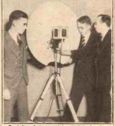
Parabolic reflectors are being tried in America behind microphones for broadcasts from large halls. So far very successful results have been obtained.
