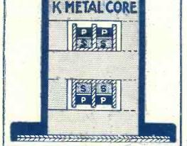
Illustration shewing "K"-METAL CORE and method of winding as employed in the "Hypermu."
