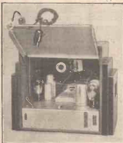
A neat hinged lid when lifted reveals the neat layout of screened components, valves and loudspeaker.
