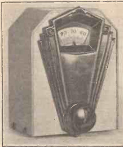
Known as the "Telexor" the Telsen extender illustrated here is completely enclosed in a metal case, and a dial light is included in its construction.
