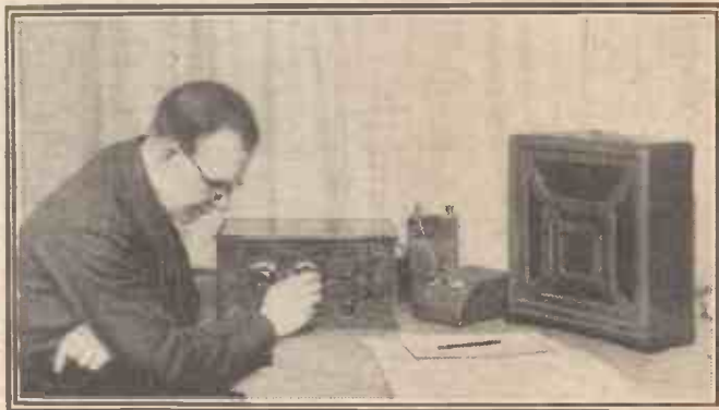
Making a final adjustment on the detector tuning dial to bring in a distant programme.
