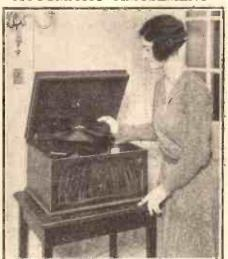
One of the most interesting modern developments is this H.M.V. unit which can be connected to practically any radio set, enabling up to eight records to be played without manual changing.
