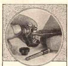
Switch springs occasionally give rise to clicking noises and poor reception owing to long use or to misuse.
