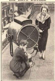
This giant loudspeaker, weighing six cwt. and mounted in a searchlight case, has been installed on a Tottenham Court Road roof by the Marconiphone Co., to relay the chimes of Big Ben to the West End.
