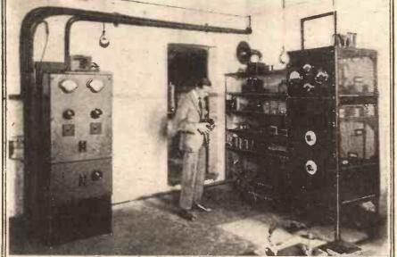
An engineer at the Johannesburg station checking up the wavelength with a small portable wavemeter. Accurate wave-keeping is not nearly so important as it is in Europe, owing to the fewer stations operating, but nevertheless the engineers always pride themselves on the accuracy achieved.
