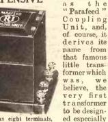
This unit has eight terminals, enabling several different circuit connections to be made.
