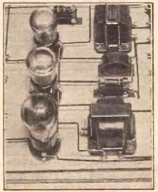
Any effort made by the home constructor to get neat, well-spaced wiring will be amply repaid by the results he obtains.
