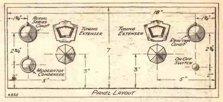
Moderator condenser. Next is the first tuning Extenser, followed by the second Extenser. This ingenious component with its automatic wave-range switching has done more to simplify radio than has any other, and rightly deserves the popularity it has
