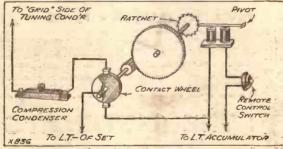
Here is the complete apparatus as described on this page by "P.W.'s" Technical Editor. Note how the metal part of the contact wheel (shaded in the diagram) is making contact with both L.T. and condenser brushes.
