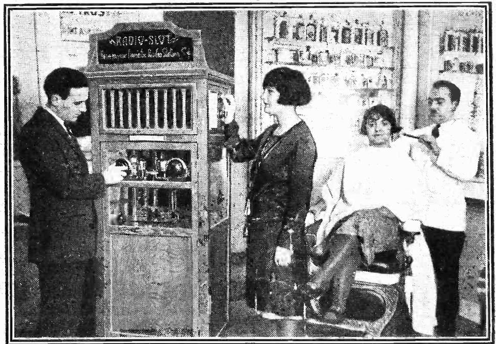
This automatic slot machine for radio programmes is being tried out in a barber's shop in Philadelphia. It is a five-valve which will work from mains or batteries, and a red light comes on as a warning about a minute before it stops, so that one can insert another coin in time to avoid missing a desirable part of some item. It should be a bit better than the usual papers that are provided to while away the time until one's turn comes to respond to "Next, please!"
