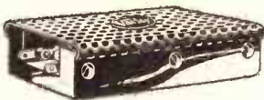
THERMAL DELAY SWITCH Specially designed for use with Osram G.U.1 rectifier. Allows filament to be run for desired time before automatically switching on the anode current. Heater circuit 4 volts and is connected across the G.U.1 filament. Price 12/6.
