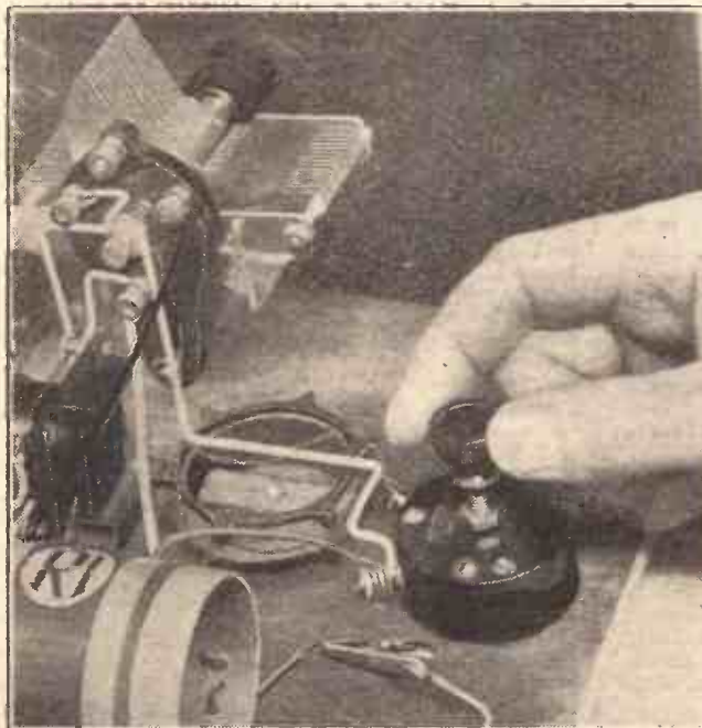
This baseboard-mounted variable condenser is operative only on the long waves, and once you have it adjusted for best results in your own local conditions you need never refer to it again.
