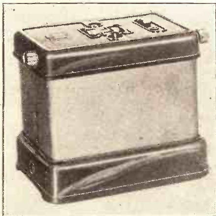
This all-mains receiver has most of its controls placed on the lid, and is quite unlike the usual British receiver of the same class.
