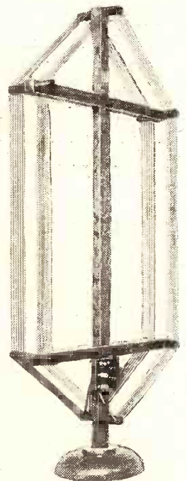
The "Elex" Frame Aerial is of the dual range variety.
