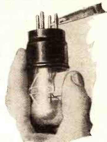
If your valve has split plugs, don't forget that they may be better for opening occasionally with a penknife.
