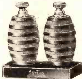
A specimen of special H.F. choke construction.
