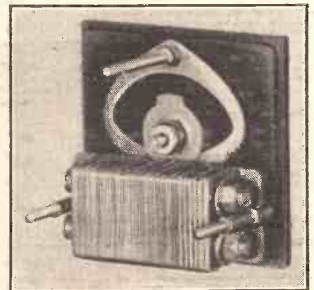
The back of the A. E. D. Volume Control with the protective moulded casing removed.
