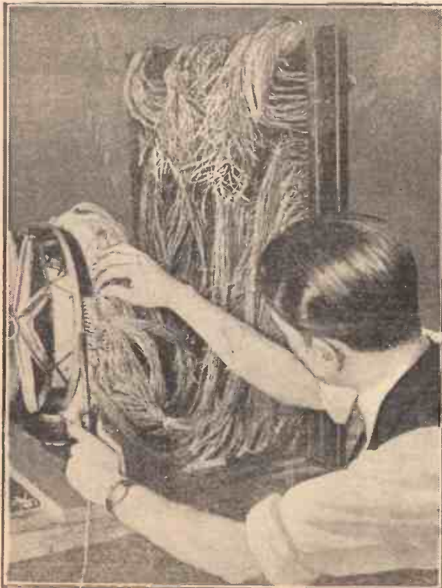
The Jenkins' television receiver includes over two thousand thin wires, joined to an equal number of photo-electric cells. It is said to be a masterpiece of mechanical ingenuity.
