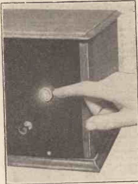
The panel-light indicates when the set is switched on, and provides ample illumination for tuning.
