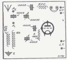
The "components" shown above are those for a simplified Reinartz one-valver, in which the primary serves both as aerial and reaction coil.
