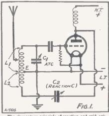
The elementary principle of reaction and grid coil , relationship is shown above.
