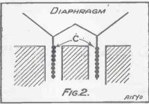
The moving coil is almost unrestricted in its up-and-down movement.
