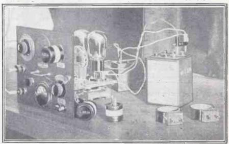
An institute has recently been inaugurated specially for the study of oscillations, and everything connected with oscillations. Here is a specially compact transmitter that is employed for producing oscillations with wavelengths of 22-38 metres.
