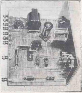
The potentiometer, which can be seen near to the earth terminal, ensures a very smooth control of reaction so that distant stations are easily received. When used with telephones dozens of foreigners will roll in, and some of them will be received at loud-speaker strength.
