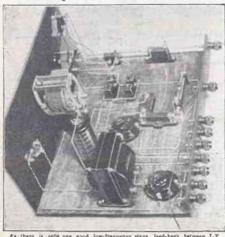
As there is only one good low-frequency stage, feed-back between L.F. valves, which is a frequent cause of poor quality reproduction, cannot possibly take place; and the set is a real dry-battery proposition.
