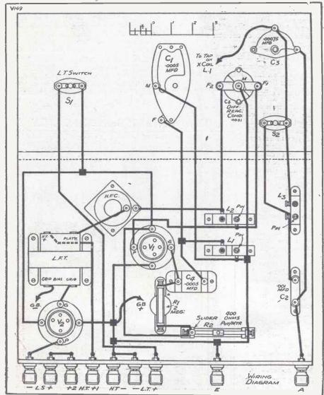
At the top of this diagram you will see a scale which represents inches, and will enable you to measure out exactly the positions of any of the components. When the wiring is completed, you should check back the connections with this diagram.
