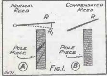
Showing how income particular unit. an improvement (B) is made on the usual reed movement (A).
