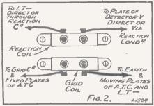
The method of connecting when both coils are wound in one direction.
