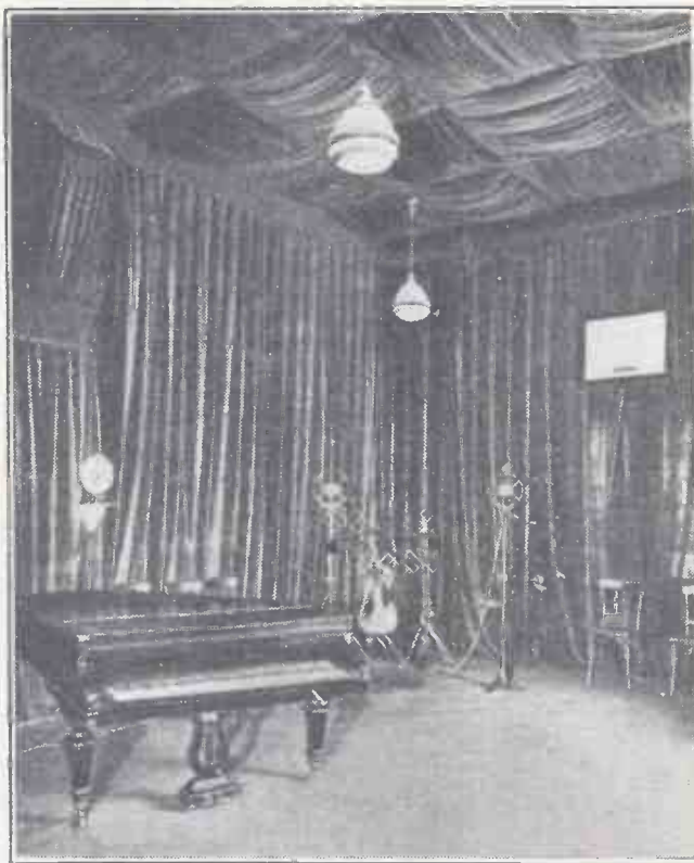
A view of the studio of the Bucharest broadcasting station which clearly shows how it is draped to avoid echo.
