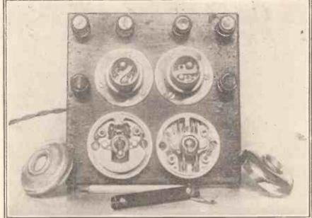
The switch covers are removed so that you can see the types of switches employed.
