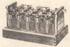
The Hart Rado, a 30-volt H.T. accumulator unit, with the capacity of 3 ampere hours.
