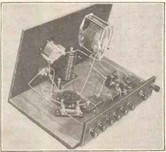
The layout is not critical, but this one was worked out rather carefully to get simple wiring and assembly and it is worth copying.
