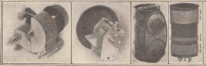
Left to right we see the following components here: The Lissen reaction condenser, a Brandes slow-motion tuning condenser, the Chakophone dual-wave range tuner, and a spar of Colvern 6-pin coils on special ribbed for
