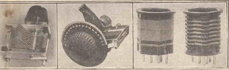
pecial Formo 6-pin dual range coil unit. The tuning components on the right hand page are, left to right, the Bowyer-Lowe reaction condenser, an Ormond slow-motion tuning condenser, traces. (The one to the right is a slot-wound long-wave coil.)
