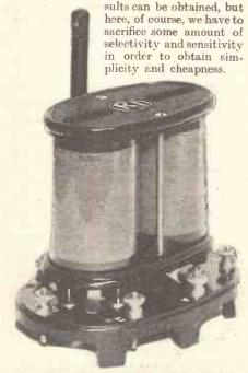
This special type of binocular coil was developed for use in their own sets by Messrs, Radio Instruments.
