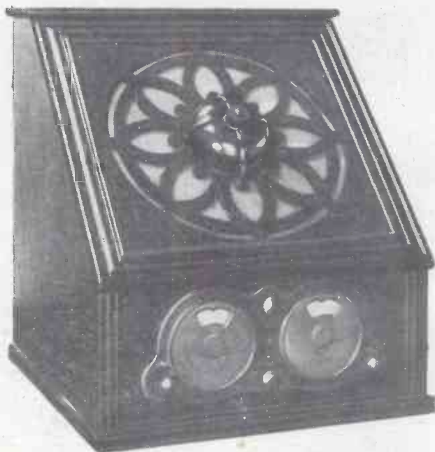
This self-contained Marconiphone set (2-valve) can be used with their A.C.4 model for all-mains operation from A.C. mains. The only external connections are aerial and earth.
