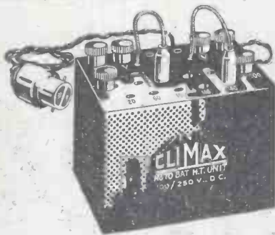
A well-known D.C. H.T. Unit. On the flex lead a plug is provided which fits a lamp socket. H.T. connections are made from the terminals, and plugs provide the various voltages.
