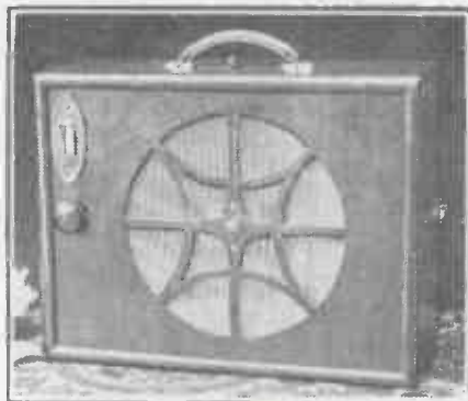
No aerial or earth need be used with the "Chakophone," though provision is made for these connections if the owner prefers to use the set in this way.
