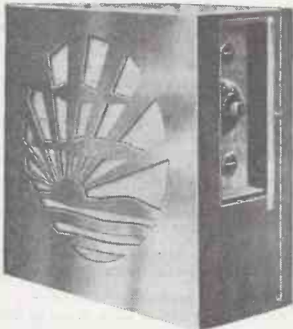
One of the best-known 5-valve sets is the Pye Portable, shown above. Both long and medium wave-lengths are covered.
