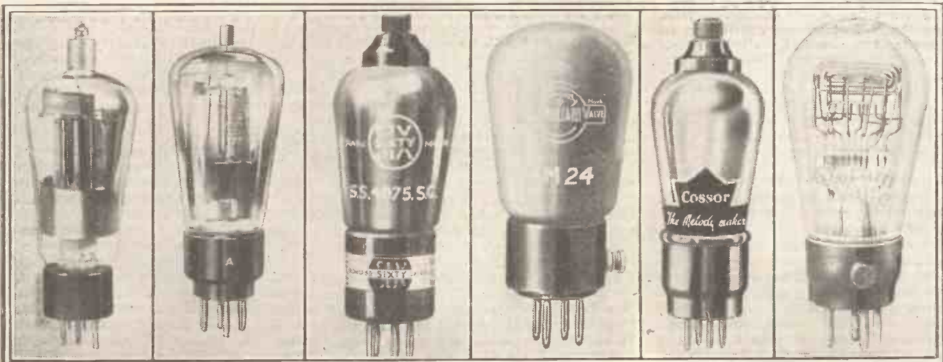
Six of the most noted multi-electrode valves. The A.C. (Mains) Cosmos screened-grid valve, B.T.-H. and Six-Sixty screened-grids, the Mullard "Pentode," Cosmos screened grid and Osram Pentode.
