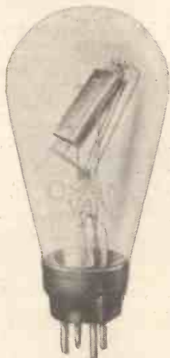
A popular power valve—the P.625, made by Osram & Marconi-Phone Cos. The impedance is 2,400 ohms and the mag. factor 6.
