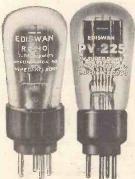
Typical examples of the Ediswan 2-volt range. That on the left is for resistance-capacity coupling, while the one on the right is a 2-volt super power valve.
