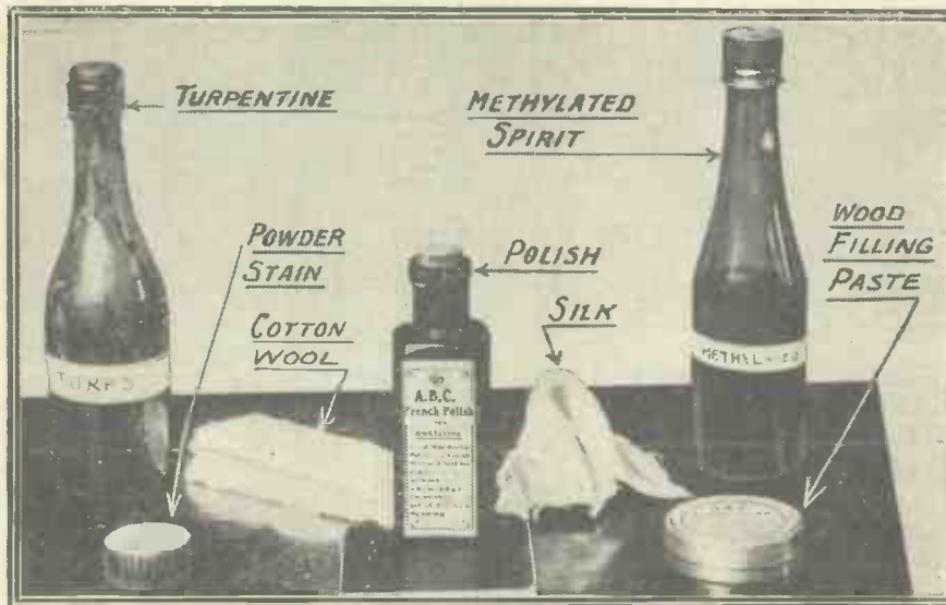
Here is the "french polishing" outfit. It is quite inexpensive and, providing you use it in the way indicated in the accompanying article, it will enable you to impart brilliant professional finishes to your radio cabinets.
