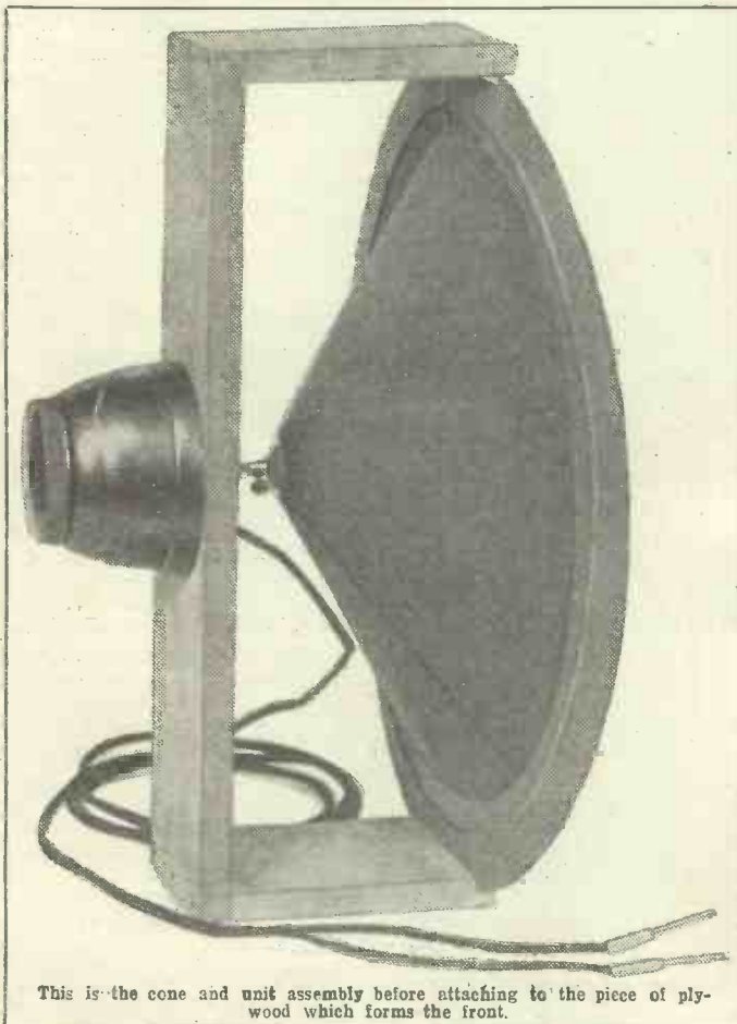
Another view at the same stage in construction as that to the left below. This shows how the driving rod is attached to the point of the cone.
