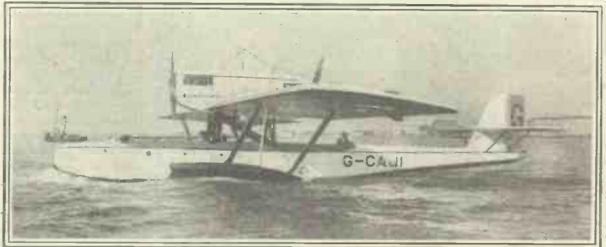
A Dornier-Napier seaplane fitted with the latest Marconi wireless transmitting and receiving apparatus. Note the aerial arranged above the fuselage.
