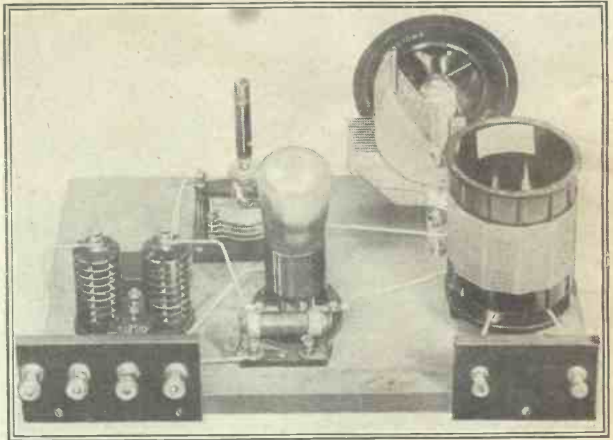
Note the absence of the grid condenser from its usual position. The wire from the tuned circuit goes direct to the grid.
