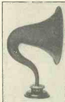
The frequencies which are necessary for speech are adequately catered for by the horn type of speaker.
