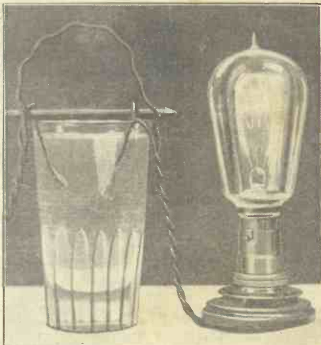
A simple way of finding the polarity of D.C. mains, which is essential if charging is to be carried out. Cut one of the wires going to a lamp socket, dip the two ends in a glass of water to which a pinch of salt has been added, and note from which wire the greater quantity of bubbles rise. This is the negative.
