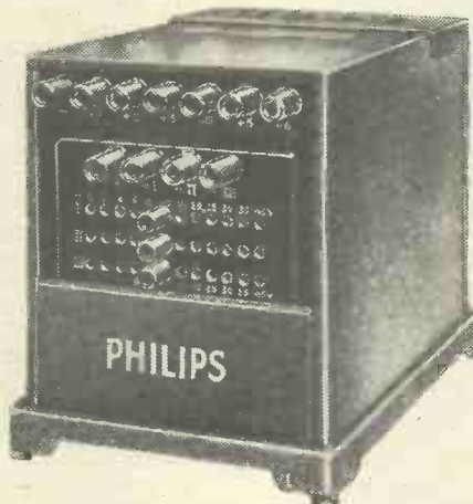
A special feature of the Philips H.T. units for A.C. mains is the very neat and safe arrangement of the plugs and sockets. These units employ valve rectification. The one illustrated is the type 3003, which gives six different H.T. voltages (up to about 200 volts) and a choice of three different grid-bias voltages ranging up to 40 volts. The price is £10 10s.
