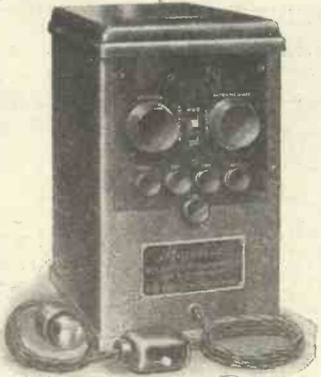
An interesting H.T. unit for use on A.C. mains is the Benjamin "Majestic" which uses a rectifying valve of the gas-filled type, without filament, and gives either a "high" or a "low" range of voltages according to the position of the small switch on the front. It is capable of giving large outputs, and is very well "smoothed." The price is £7 15s.
