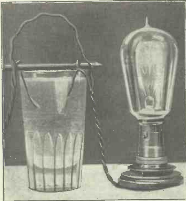
A simple way of finding the polarity of D.C. mains. Cut one of the wires going to a lamp socket, dip the two ends in a glass of water to which a pinch of salt has been added, and note from which wire the greater quantity of bubbles rise. This is the negative.
