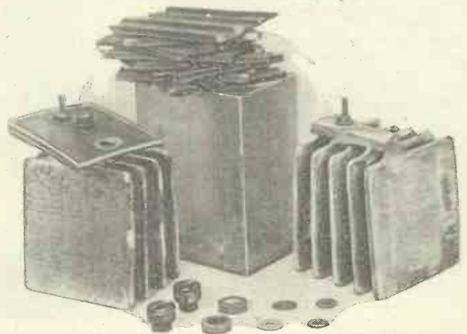
Apart from the electrolyte or "acid," an ordinary accumulator merely consists of a containing case with cover, two sets of plates with separators, and the connecting terminals, nuts, etc. (Generally there is one more negative plate than positive.)
