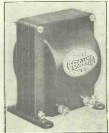
The Ferranti L.F. choke, type B1, sells at 21s. It has an inductance of 20/40 henries, according to the D.C. load, and a D.C. resistance of 500 ohms.
