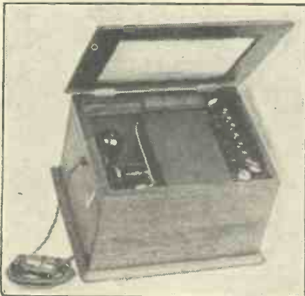
One of the Burndep't range of mains units. The photo shows one of the first introduced by this firm, namely, the Universal Heavy Duty model, which gave currents up to 40 milliamps at voltages up to 180. Price, £9 17s. 6d.
