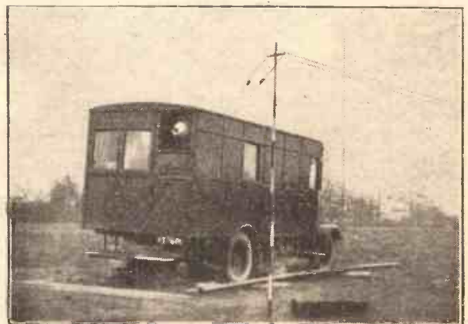
The Daimler van housing the 2 kw. transmitter used by the B.B.C. in the "regional" tests in the North of London. Note the huge insulator and the twin wires leading to the separate insulator beneath the aerial itself.
