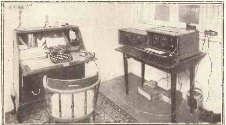
This photograph shows the receiving apparatus at 2DA—"P.W.'s" experimental station—which is described in detail in this issue. Messages picked up in the 'phones are typed direct as received. The Morse key and switch on the bureau control the transmitting apparatus, which is situated at some distance from the receiver.
