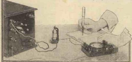
A reading being taken with a milliammeter and resistance, as described in the accompanying article.
