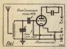
there is no signal—determines, to a large extent, the effectiveness of the valve as a detector. The grid current which flows is controlled by the voltage of the grid with respect to the filament, and the majority of valves require that the return end of the grid leak be slightly positive, with respect to the negative side of the filament.
