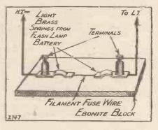
ebonite strip, and thus place a fuse in the anode supply to every valve. Such a device is particularly useful to the experimenter, whether he works with a battery eliminator, with dry batteries, or H.T. accumulators.
