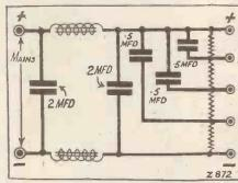
The above diagram is supposed to represent the connections of an H.T. Battery Eliminator, for use on D.C. mains, but it is wrong and would not work properly.
