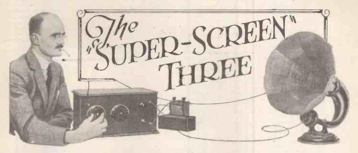
'HE introduction of the screened grid valve has placed the designer of sensitive long-distance sets in a somewhat difficult position, since these valves bid fair to effect something like a revolution in the results which can be expected from a given number of H.F. stages, and in our methods of H.F. am-
