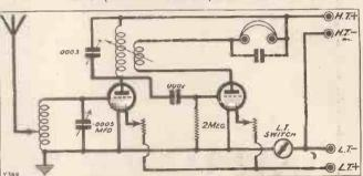
The correct connections for an H.F. and Det. receiver are shown above. In the "What is Wrong?" diagram last week the filament switch did not control both valves, the aerial condenser was '005 mfd. instead of '0005, and the grid leak was taken to H.T. + instead of to the filament circuit.
