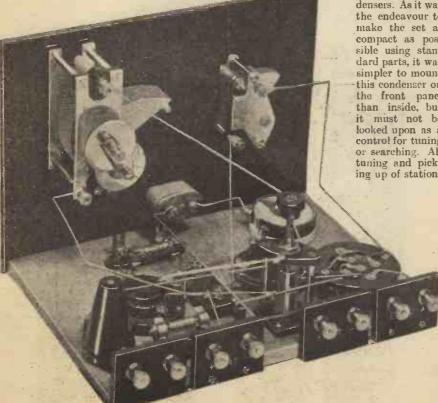
2'de terminals are grouped in pairs on separate terminal-strips—a point which greatly simplifies connecting-up and reduces the danger of placing the wrong battery leads on the wrong terminals.
