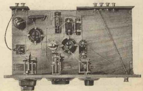
The bigh-frequency components are well spaced out and the leads widely separated. The three devibles can be seen clearly.
