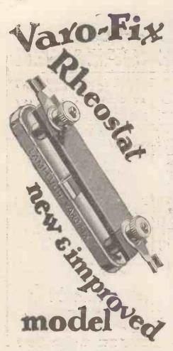
This is the Rheostat that everyone will use. It is built upon an aluminium base which carries a special spring slider, making a positive contact with the resistance element, which is removable, and can be replaced with others of different value. It is very compact, occupies but little space, and can be put near to valveholders, thereby reducing the wiring—a desirable feature in modern Radio Receivers.
