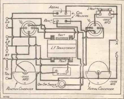
The correct connections for a Det. and L.F. receiver are shown above. In the "What is Wrong?" diagram last week there was no H.T. to the 1st valve, and no H.F. Choke. The 'on-off" was connected across the L.T. battery, and the Grid Bias plus should have been taken to L.T. minus. (Another "What Is Wrong?" diagram will appear next week.)
