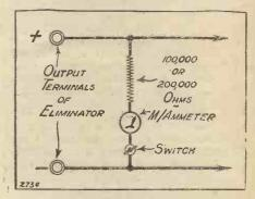
Briefly, the method is this: A high resistance of accurately known value is connected across the H.T. terminals, and in series with this is placed a milliammeter with a suitable scale to measure the current flowing. Then, by the simple application of Ohm's Law the voltage can be determined, the arithmetic involved being of a trifling nature if the value of the high resistance has been wisely chosen.
