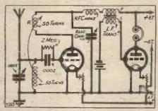
The correct connections for a Detector and L.F. receiver with condenser-controlled reaction are shown above
