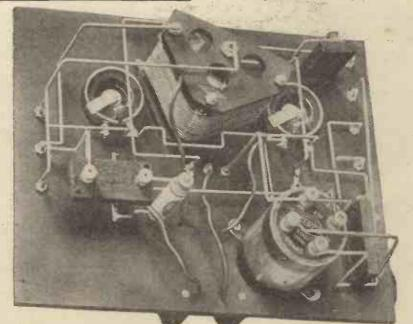
The earlier reflex receivers incorporated very straightforward circuits. The one above merely had a crystal detector and primary of an L.F. transformer connected across an anode-tuning coil. The secondary of the transformer was included in the grid circuit of the valve.
