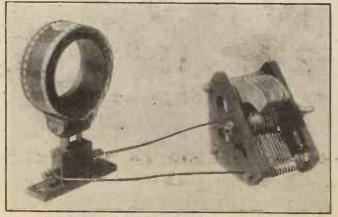
Just a coil and condenser forms the simplest kind of H.F. intervalve coupling circuit.
