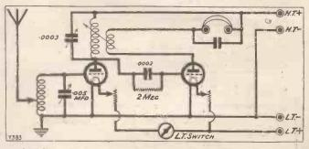
The above diagram is supposed to represent the connections of an H.F. (Tuned Anode) and Det. receiver. But it is wrong and the set would not work.
