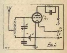
When we come to the anode rectifier, you will find it of the greatest importance to provide a more or less exact adjustment of either the grid bias or the anode voltage. In this method of rectification, a sufficient negative grid bias is given to the detector to prevent grid current, and one part of the incoming signal alters the anode current while the other does not.
