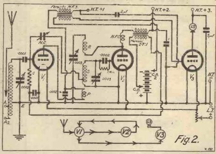
of course, going to the tuning condenser and the grid condenser and leak. It is important to join the primary correctly, and the anode of  $V_1$  should be connected to the bottom of the coil.
