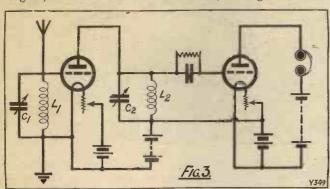
we must provide some sort of output circuit in the anode circuit of our H.F. valve, in order that it may amplify properly and also give us our amplified signals in a form which will be most effective for applying to the detector which follows.
