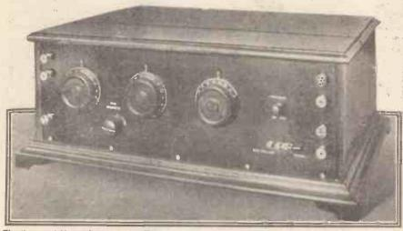
The three variable condensers (aerial, H.F. and reaction) have vernier dials, while a losser control is provided for cutting down the volume when necessary.
